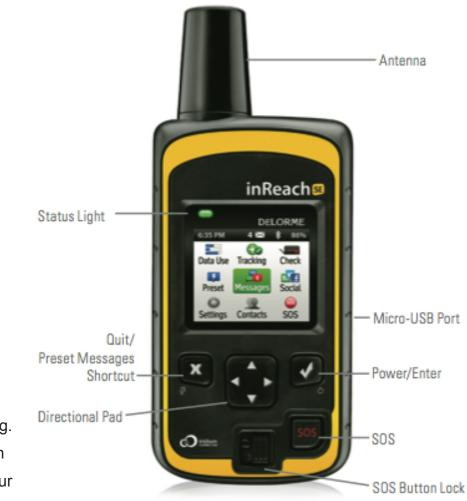
**Antenna** - Keep the satellite communicator antenna pointing up toward the sky and the face of the device pointing away from your body.
