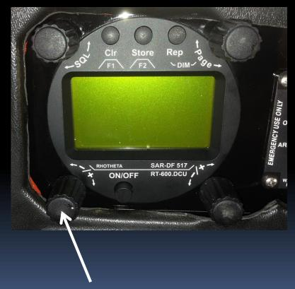
Volume is controlled by the rotary switch here
