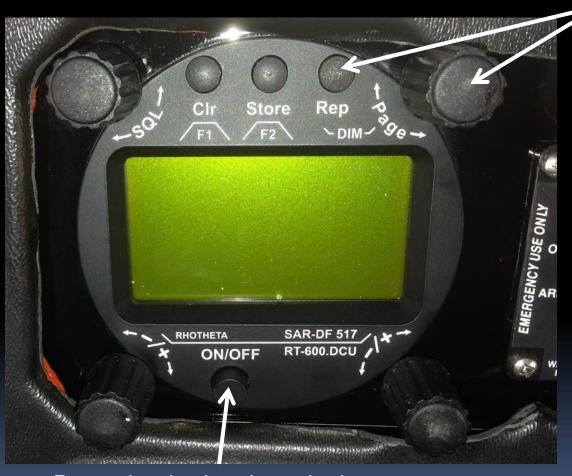
Power is wired to the avionics master but if the unit does not come on PRESS ON/OFF
