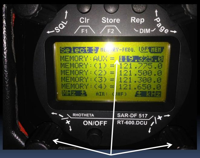
To DF any frequency turn the Page rotary knob to MEM and use the two lower knobs to change the frequency in AUX
