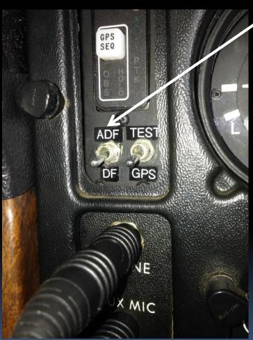
To listen to the RT-600 put the ADF/DF switch in the DF position and activate the ADF switch on the intercom panel.
