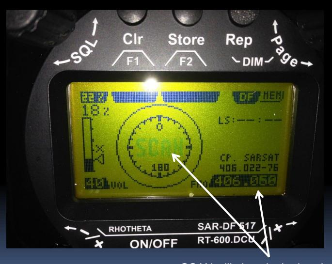
SCAN will show in the bearing window along with the channels being scanned
