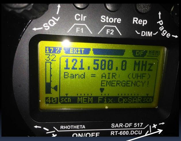
Select a frequency by turning the rotary knob. Cycles through SCN (Marine), MEM, FIX (121.5, 156.800 Marine Ch 16, 243.0), and CpSAR, SCN (CpSAR)
