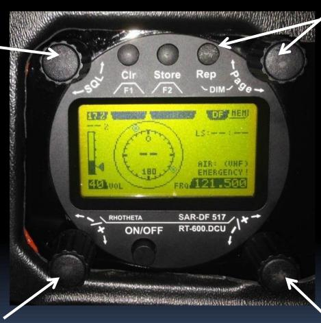
Rotary switch selects pages and dims display if DIM button is pressed first
