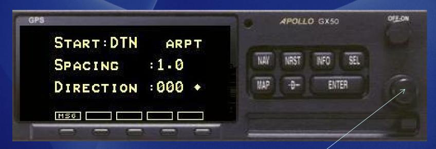
Turn SMALL KNOB to change the track spacing (0.2 – 5.0 NM)
