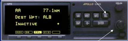
Turn Outer Knob to the desired flight plan
