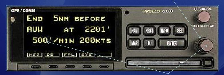
Use the Small Knob to change the descent rate from 100' – 5,000'/minute in 10'/minute increments
