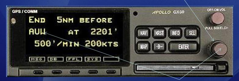
By turning the Small Knob you may select any of the waypoints in the active flight plan
