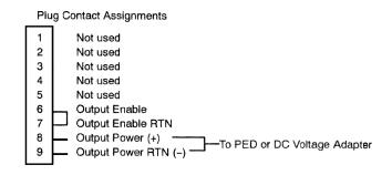
Figure 3. Mating Plug Wiring
